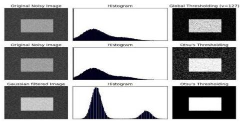
Fig 3: global thresholding with noisy image, Otsu's thresholding with noisy image and Otsu's thresholding with Guassian filtered image
